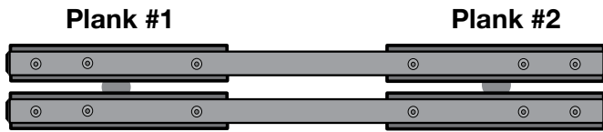
Front view of stand-alone platform for a single cabinet. Set-up consists of two planks and four connectors.
