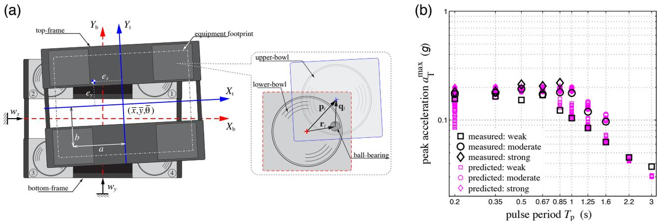
**Figure 1:** (a) Rolling isolation system geometry and notation [7]. (b) Measured and predicted response of a heavily-damped rolling isolation system [8].
